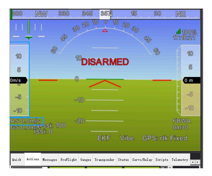
• Hold the pitot tube with your hand and blow air into the pitot tube. If the airspeed value changes according to the airflow speed, the inspection is complete.
